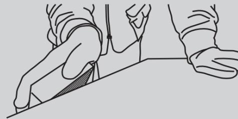
Edges can be finished by using sanding discs fitted onto hand held angle grinder. The same result can be obtained by hand using abrasive diamond sponges or emery paper. With a light passage on the side of the slab, you can obtain a slightly rounded-off edge or with repeated passages a bevelled effect.
