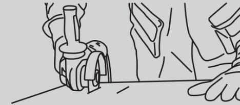
All products of Neotra can be cut using diamond discs fitted onto the hand-held electrical grinding machine. In this case, the SLAB will have a cleaner and better defined edge than by cutting and breaking the SLAB.
